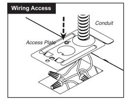
Make all electrical connections to the fixture. Attach wiring access plate cover.
